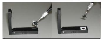
Examine the anti-static suction tip for particulate before use. Clean with an alcohol wipe as necessary.
