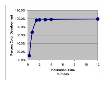
Graph depicts results obtained with the P4900 unit set to temperature of 58.5°C for various time periods plotted as a percent of B3 dosimeter color development compared against the results obtained from a 15 minute 58.5°C Fisher box air incubator cycle.
