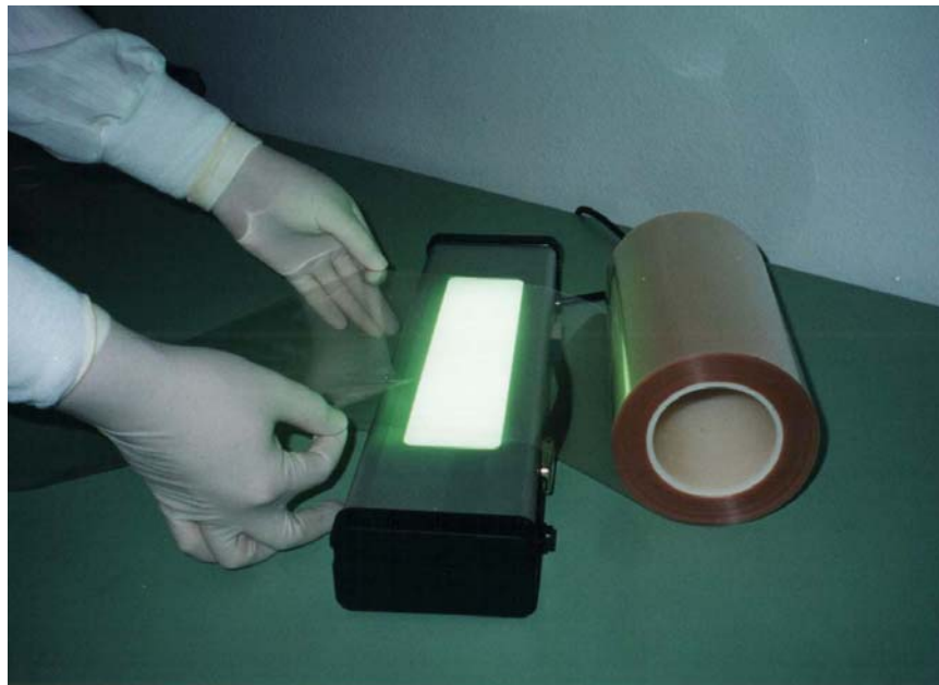
200 meter long 200 mm wide B3 film roll prior to final film roll slitting
